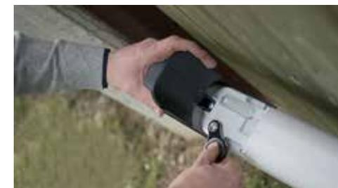
Possibility to unlock motor with transmitter
