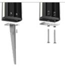
Simplified installation using garden spike or anchor plate
