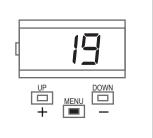
Press the MENU button for 1 second to display the parameter in order to save the modified value, or MENU quickly to quit the function without saving.
