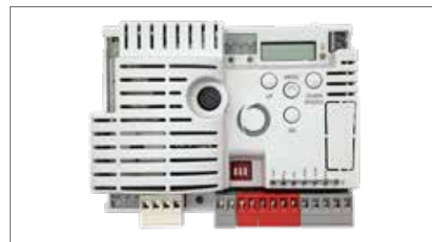
CT10224 control board with integrated receiver
