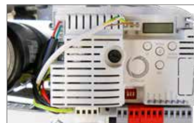
CT102 24 control board with integrated receiver
